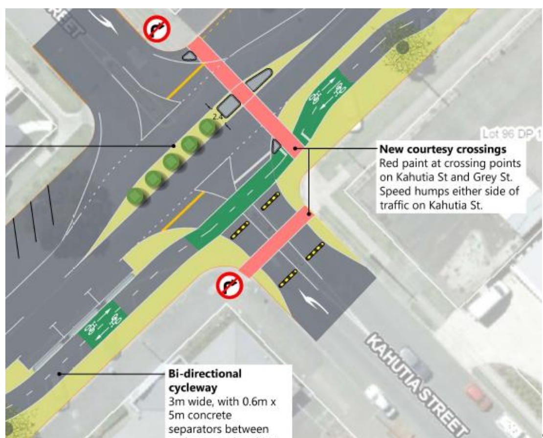
Figure 5.3-11 – Proposed layout at the Grey Street/Kahutia Street intersection (extracted from the design)
