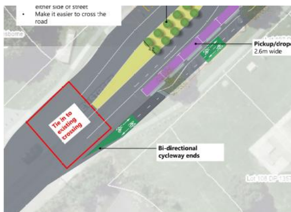
Figure 5.3-18 – Missing tie-in details
