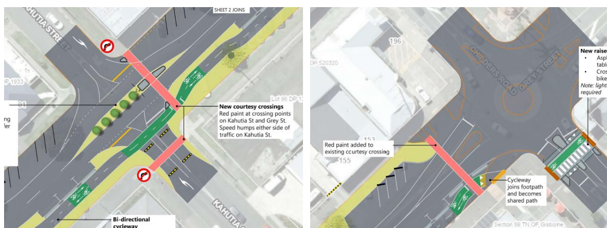
Figure 5.3-6 – Proposed courtesy crossings (extracted from the design)
